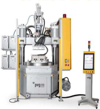
VERTICAL INJECTION MOULDING MACHINE WITH 4 PISTONS, TOP-BOTTOM MOVEMENTS AND VERTICAL INJECTION UNIT EQUIPPED WITH A LOWER ROTATING TABLE WHERE TWO HALF-STAMPS ARE LOCATED
